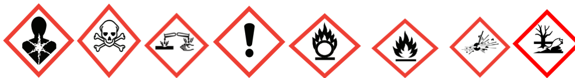
Serious health Risk Acute Toxicity Corrosive Health hazard Ozone hazard Oxidising risk Flammable Explosive Dangerous to enviroment
